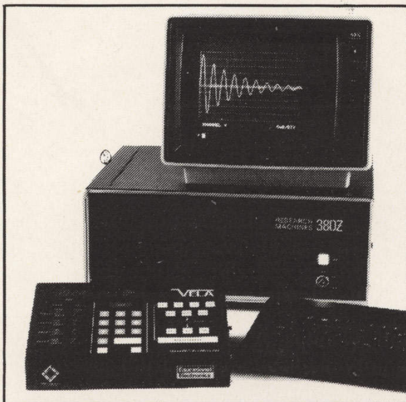
The educational electronics VELA acting as an 'intelligent' interface to a 380Z microcomputer.
