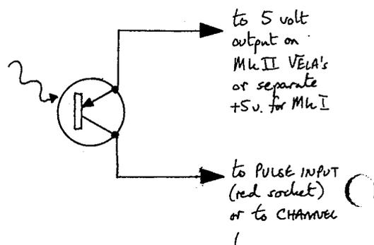
THIS WORKS RELIABLY FOR PHOTODIODE R.S. 305 - 462<sup>†</sup> AND I.R. DETECTOR R.S. 306 - 083<sup>†</sup> PROVIDED THEY ARE WELL SHIELDED FROM EXTRANEIOUS LIGHT AND THAT THE CARD, etc. USED TO CUT THE LIGHT BEAM IS TRULY OPAQUE.
