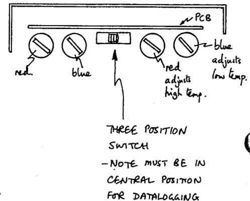
ACCURACY:  $\pm 0.5^{\circ}\text{C}$  IN RANGE  $0^{\circ}\text{C}$  TO  $70^{\circ}\text{C}$ ,  $\pm 1^{\circ}\text{C}$  EITHER END OF RANGE.
