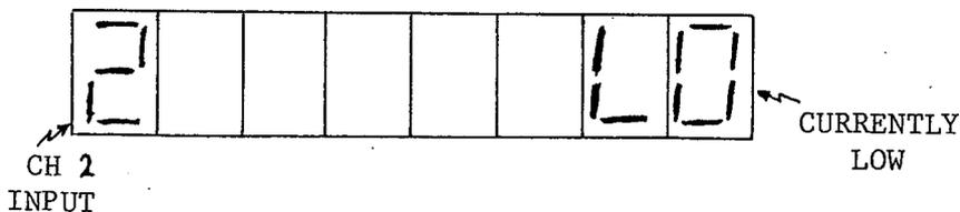
(BOTH CH 1 INPUT AND CH 2 INPUT ARE PROGRAMMED TO BEHAVE AS SCHMITT TRIGGER INPUTS TO IMPROVE PERFORMANCE RELIABILITY.)
