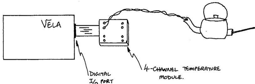
FILL A KETTLE WITH COLD WATER. POP SENSOR INTO KETTLE VIA SPOUT, BUT DO NOT REST ON ELECTRIC HEATING ELEMENT. KEYPRESS SEQUENCE
