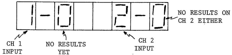
WHEN ONE OF THE LIGHT BEAMS IS INTERRUPTED THE HYPHEN IS CLEARED. WHEN THE LIGHT BEAM IS RESTORED THE HYPHEN RETURNS AND THE RESULT TOTAL FOR THAT INPUT IS INCREMENTED e.g.
