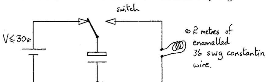
THE CAPACITOR IS DISCHARGED THROUGH THE WIRE CAUSING HEATING OF THE WIRE. THE RESULTANT TEMPERATURE RISE CAN BE USED TO DETERMINE THE ENERGY TRANSFERRED FROM THE CAPACITOR AND THUS TO DEMONSTRATE  $\text{ENERGY} \propto V^2$ . THE ENERGY TRANSFER IS  $\sim 50\%$  EFFICIENT.
