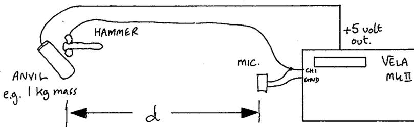
SET EXTERNAL/INTERNAL SWITCH TO INTERNAL, AND CH1 TO  $\pm 250$  mV.
