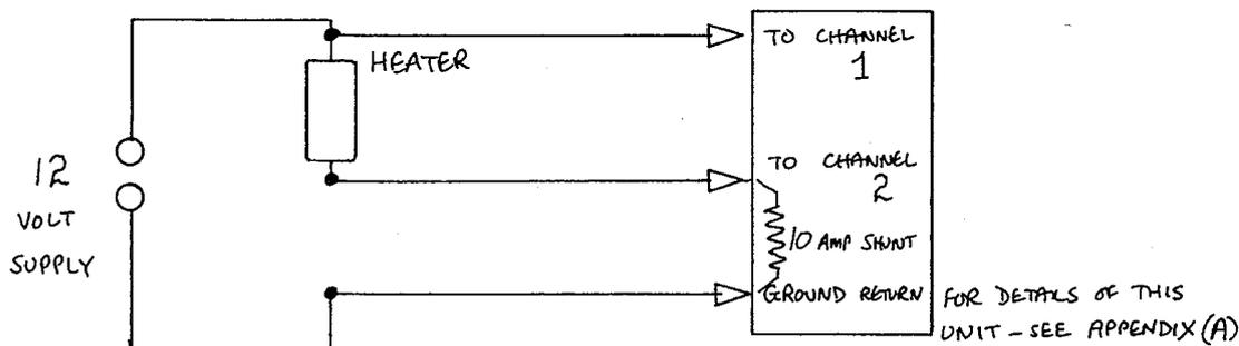
SET CH 1 INPUT TO  $\pm 25V$ , CH 2 INPUT TO  $\pm 250mV$ .
