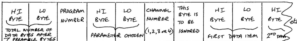
NOTE THAT THE FORM OF THE DATA IS DIFFERENT. UP TO 1024 DATA BYTES ARE TRANSFERRED. 2 DATA BYTES ARE NEEDED FOR EACH RESULT. THE TEMPERATURE RESULT IS OBTAINED AS FOLLOWS:-
