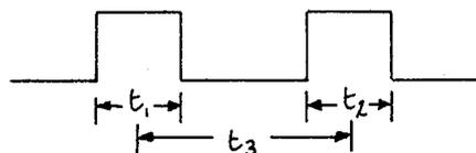
VELA CALCULATES SPEEDS CORRESPONDING TO  $L/t_1$  AND  $L/t_2$ .
