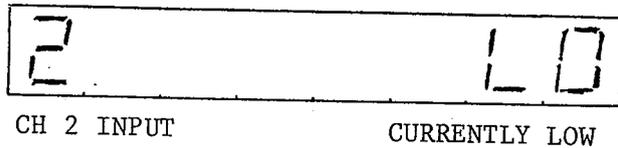
(BOTH CH 1 INPUT AND CH 2 INPUT ARE PROGRAMMED TO BEHAVE AS SCHMITT TRIGGER INPUTS TO IMPROVE PERFORMANCE RELIABILITY.)
