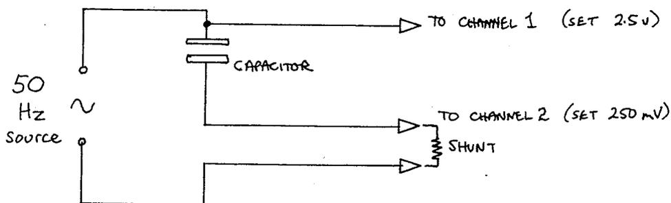
CHANNEL 1 MEASURES VOLTAGE, CH2 MEASURES CURRENT (SEE APPENDIX A). A SHUNT OF 1mA IS SUITABLE AND VELA INDICATES THE PHASE LAG OF CURRENT COMPARED TO VOLTAGE, i.e. 270 DEGREES (EQUIVALENT TO CURRENT LEADING VOLTAGE BY 90 DEGREES). USE OF A TWIN BEAM OSCILLOSCOPE PROVIDES VISUAL SUPPORT FOR THE MEASUREMENT.
