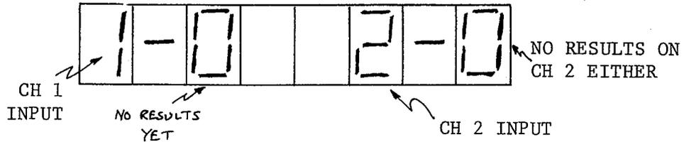
WHEN ONE OF THE LIGHT BEAMS IS INTERRUPTED THE HYPHEN IS CLEARED. WHEN THE LIGHT BEAM IS RESTORED THE HYPHEN RETURNS AND THE RESULT TOTAL FOR THAT INPUT IS INCREMENTED, e.g.
