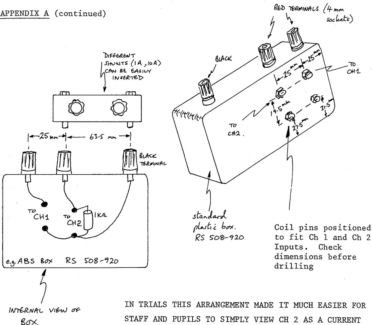
IN TRIALS THIS ARRANGEMENT MADE IT MUCH EASIER FOR STAFF AND PUPILS TO SIMPLY VIEW CH 2 AS A CURRENT RANGE. THE 1k $\Omega$  RESISTOR REPLACES THE 1000  $\Omega$  METER. THE BASIC BOX WITHOUT ADDITIONAL SHUNTS CORRESPONDS TO A CURRENT OF 100  $\mu$ A. YOU ARE ADVISED TO AVOID USE OF DUAL RANGE SHUNTS, AS THESE CAN GIVE FALSE RESULTS BECAUSE OF THE COMMON NEGATIVE USED BY CH 1 AND CH 2 INPUTS.
