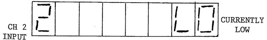
(BOTH CH 1 INPUT AND CH 2 INPUT ARE PROGRAMMED TO BEHAVE AS SCHMITT TRIGGER INPUTS TO IMPROVE PERFORMANCE RELIABILITY.)
