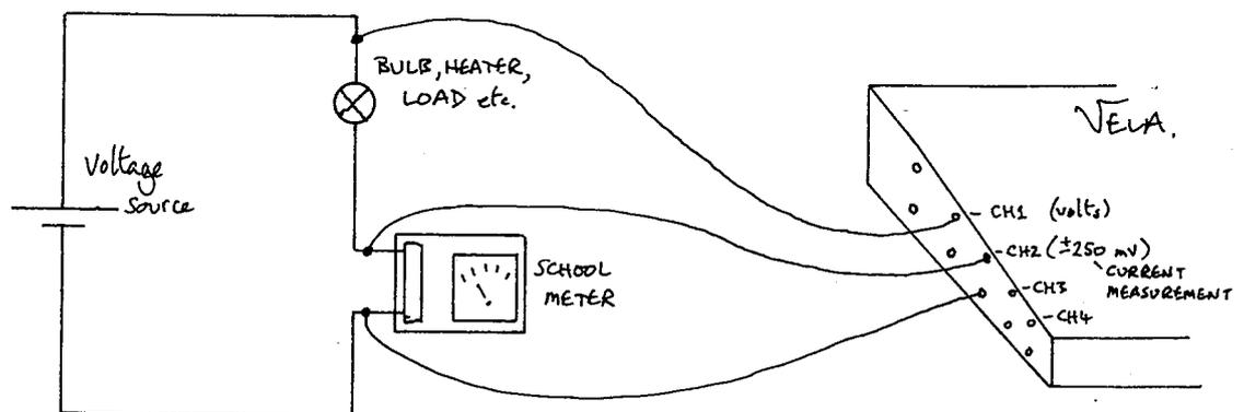
THIS SIMPLE APPROACH OF LITERALLY MEASURING THE VOLTAGE ACROSS THE METER RESULTS IN COMPLICATED WIRING AND IT IS SUGGESTED THAT A SIMPLE PLUG-ON UNIT BE CONSTRUCTED FOR VELA, e.g. IF YOU USE A UNILAB 1000  $\Omega$  METER.
