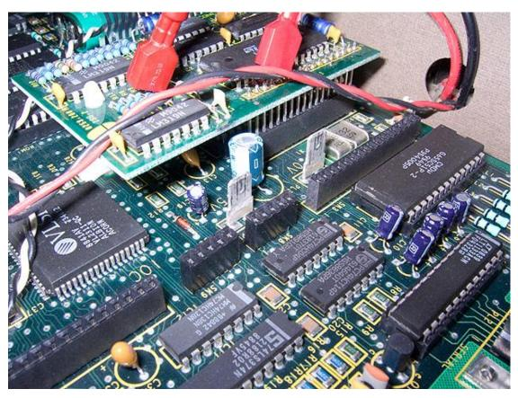
11. Connect the supplied power cables to the motherboard and then the PSU power cables to the piggy back connectors.
