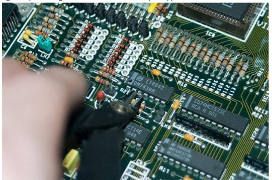
5. Fit the supplied 14-way socket in the position of IC9 noting the orientation of the socket when placing it on the motherboard.
