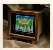
The Touchtech 501 can be added to any of the metal cabinet monitors and used with the BBC 'B' or 'Master' series of computers and the wealth of 'special needs' and general software that is readily available. The touchscreen uses infrared technology with a resolution of 120H x 90V.
